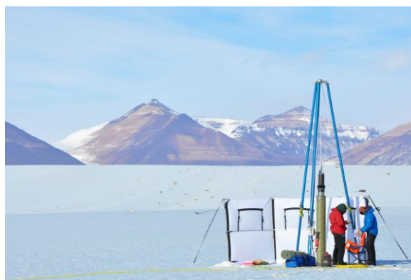
Scientists are drilling a large-volume ice core on the Taylor Glacier ablation zone, Antarctica. Bubbles in the ice at the site contain evidence of ancient atmospheric composition. The Blue Ice Drill is an easily-transportable drill developed by IDDO that is capable of retrieving cores of approximately 9.5 inches in diameter up to 15 meters in solid ice. Credit: Jeff Severinghaus.
