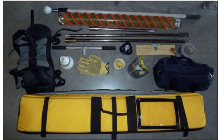
IDDO hand auger kit contents. For more information about the IDDO hand auger kit, visit: http://www.icedrill.org/equipment/
