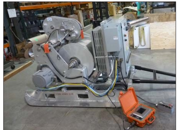
The new deep logging winch for logging boreholes up to 4000 meters deep.
