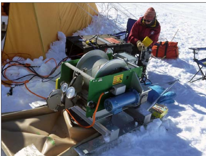
The new intermediate logging winch for logging boreholes up to 1500 meters deep.
