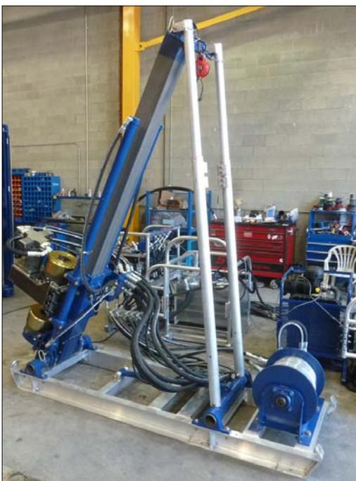
*The new minerals exploration drill rig for the ASIG Drill system.*
