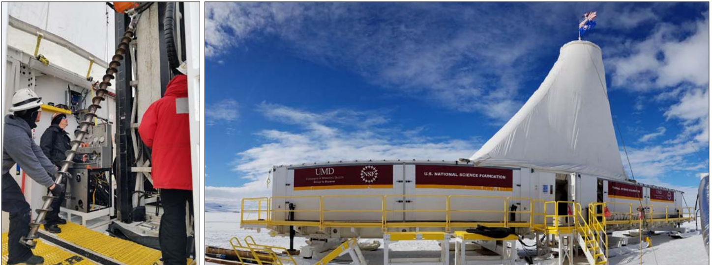
Loading the 10-foot-long auger stem onto the Rapid Access Ice Drill (RAID) (left). Exterior view of the RAID system (right). Credit: Jay Johnson
