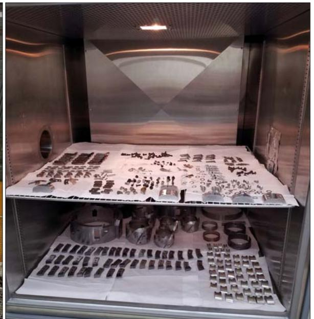
*Left: Ultrasonic cleaning of cutters and other metal parts. Right: Baking of drill parts in a Tenney environmental chamber at 50 °C. Credit: Jay Johnson.*
