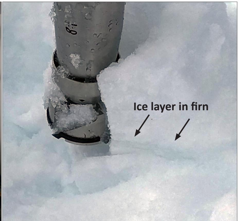
*Left: RAM Drill sonde testing in Madison, Wisconsin. Right: RAM Drill testing at Raven Camp, Greenland. Ice layers in the firn were evident both visually and in drilling. Credit: Chris Gibson.*
