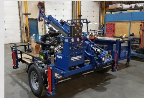
Example of BASE Drill rig, platform and control station
