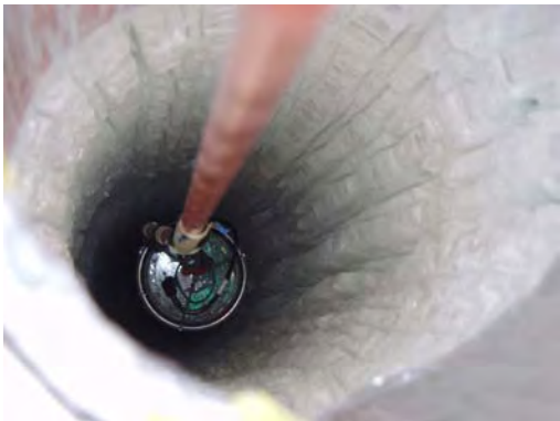
A Digital Optical Module (DOM) is lowered into a hole in the ice at Amundsen-Scott South Pole Station as part of the IceCube project. IceCube will search for neutrinos from distant astrophysical sources. Photograph Credit: Ethan Dicks, National Science Foundation.
