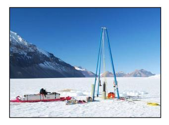
Blue Ice Drill –An agile drill capable of retrieving cores of approximately 9-1/2 inch diameter to depths up to 25 meters in solid ice. The drill, developed for the University of California at San Diego, was used with great success to collect samples of "blue ice" on Taylor Glacier during the 2010-11 and 2011-12 Antarctic field seasons.
