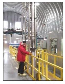
its main-hole drilling on New Year's Eve after five production seasons. The drilled depth as of January 1, 2012, is 3405 meters. The DISC Drill will remain at WAIS Divide for replicate coring in 2012-13.
