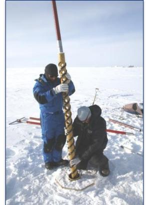
Hand augers are typically operated by the investigator without assistance from IDDO drillers.
