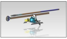
Intermediate Depth Drill (IDD) - Many of the coring objectives given in the Long Range Science Plan, such as those in the IPICS 2k array and 40k network, are attainable in many locations with an intermediate-depth drill, meaning one that can collect core from a fluid-filled hole down to a depth of 1500 meters. IDDO
