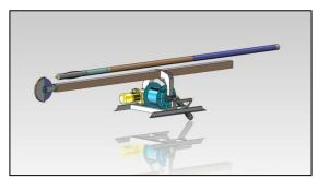
Intermediate Depth Drill (IDD) - Many of the coring objectives outlined in the Long Range Science Plan, such as those in the IPICS 2k array and 40k network, are attainable in many locations with an intermediate-depth drill, meaning one that can collect core from a fluid-filled hole down to a depth of 1500 meters. IDDO
