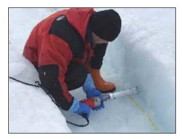
**Chipmunk Drill** – The smallest drill in the IDDO inventory, it is a hand-held, motor driven coring drill that collects 2-inch diameter cores in solid ice. It has two barrels, one 15 cm long and one 50 cm long. The drill has been used on one project (for which it was designed) at Pakitsoq, West Greenland, in 2003 and 2004, and for several demonstrations of ice coring for the public in the U.S.
