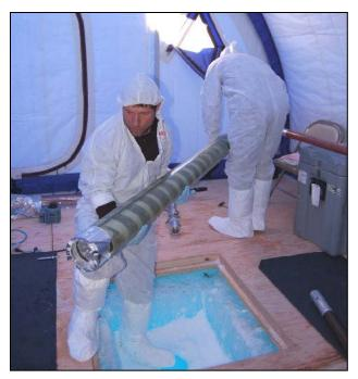
**Prairie Dog** – A modification of the hand auger, the Prairie Dog includes a stationary outer barrel that allows operations in solid ice as well as firn. Limit of depth of use is approximately 40 meters (with a Sidewinder, *q.v.*). The drill has been used almost exclusively by Jay Kyne, its designer, who is a part time driller/engineer with IDDO.
