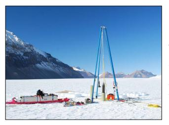
**Blue Ice Drill (BID)** – An agile drill capable of retrieving cores of approximately 9-1/2 inch diameter to depths up to 30 meters in solid ice. The drill, developed for the University of California at San Diego, was used with great success to collect samples of "blue ice" on Taylor Glacier during the 2010-11 and 2011-12 Antarctic field seasons. Modifications to the drill for use in firn were tested successfully in Greenland in 2013.
