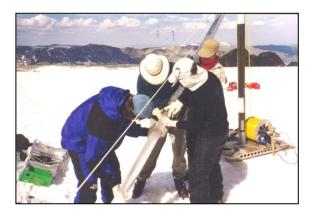
**Electrothermal Drill** – This drill melts an annulus around the core. It supplements the 4-Inch drills and can be substituted for the 4-Inch sonde, using the same winching system, for use in ice warmer than about minus 10° C. It takes a 3-inch core. It is particularly useful in ice close to the pressure melting point, where electromechanical drills suffer risk from melting and refreezing of the ice. Much
