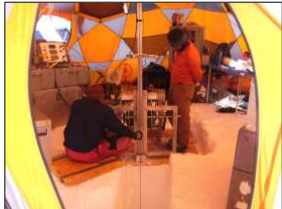
Scientific drilling on the Mt Hunter Plateau of Denali provides a 1,000 year record of precipitation and atmospheric circulation in Central Alaska. Drilling at this site was accomplished by wind and solar energy without the need for gas-fueled generators. Credit: a) Seth Campbell, CRREL; b) Dom Winski, Dartmouth
