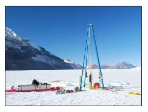
2.1.5 Blue Ice Drill (BID) – An agile drill capable of retrieving cores of approximately 9-1/2 inches (241mm) in diameter. The BID system had a depth capability of 30 m in solid ice in its original design. The drill, developed for the University of California at San Diego, has been repeatedly used with great success to collect samples of 'Blue Ice' on Taylor Glacier each season since its initial deployment during the 2010-2011 field
