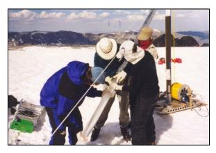
**2.1.9 Electrothermal Drill** – The Electrothermal Drill melts an annulus around the ice cores it collects. It supplements the 4-Inch Drills and can be substituted for the 4-Inch Drill sonde, using the same winch systems, for use in ice warmer than about minus 10 °C. The drill collects a 3-inch core. It is particularly useful in ice close to the pressure melting point, where electromechanical drills are at risk from melting and refreezing of the
