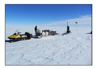
**2.1.11 Small Hot Water Drills** – The IDDO Small Hot Water Drills (SHWD) use hot water to create shallow holes in the ice. They are non-coring. Primary use is for shot holes for seismic work, but they have also been used for access holes through a thin ice shelf. These drills are transportable by light aircraft and helicopter. These systems have typically been operated by investigators without assistance from IDDO drillers.
