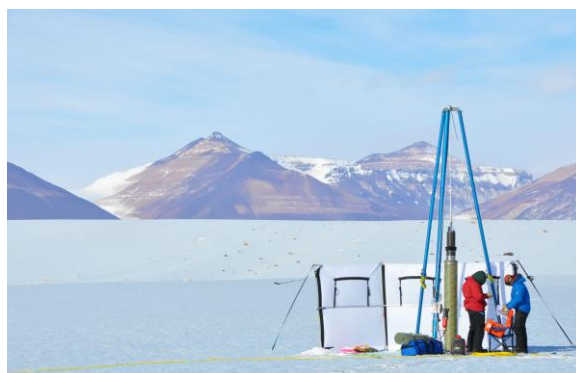
Scientists are drilling a large-volume ice core on the Taylor Glacier ablation zone, Antarctica. Bubbles in the ice at the site contain evidence of ancient atmospheric composition. The Blue Ice Drill is an easily-transportable drill developed by IDDO that is capable of retrieving cores of approximately 9.5 inches in diameter up to 15 meters in solid ice. Credit: Jeff Severinghaus.
