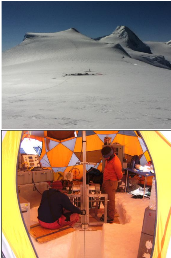
Scientific drilling on the Mt. Hunter Plateau of Denali provides a 1,000-year record of precipitation and atmospheric circulation in Central Alaska. Drilling at this site was accomplished by wind and solar energy without the need for
