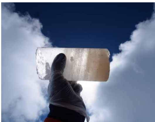
Part of an ice core retrieved from Mt Hunter Plateau of Denali exhibits layering and dust carried to the area from afar. Credit: Brad Markle, Univ. Washington.
