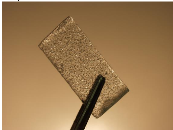
The bubbles visible in this piece of ice from an Antarctic ice core contain carbon dioxide and other gases that were trapped in the ice when formed many thousands of years ago. Ice cores provide the only natural archive of ancient air. Credit: Oregon State University .
