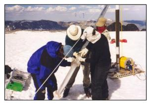
success. The sonde is particularly useful in ice close to the pressure melting point, where electromechanical drills are at risk from melting and refreezing of the surrounding ice. The Thermal Drill has performed well in British Columbia, Alaska and in southeastern Greenland. The drill was most recently used to drill through firn aquifer layers in SE Greenland during spring 2013 and spring 2015.
