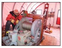
knocking sound witnessed in the field, an oil change, addition of adjustable leveling screws between the winch and sled frame, creation of a reference guide for operation of the LCI-90i display (tension settings, depth zeroing, field calibration), and determination of a method to record tension from the LCI-90i.
