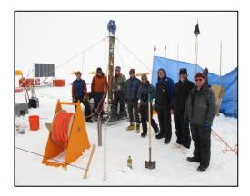
The 4-Inch Drill was most recently used in conjunction with field testing of the Rapid Access Ice Drill (RAID) system outside of McMurdo Station near Minna Bluff during the 2017-2018 Antarctic field season. A 131-meter core of good quality was drilled and firn-air samples were collected from nine separate depths. The drilling effort also aided in determination of the depth of the firn-ice transition at the site, providing valuable data for the nearby RAID field testing operations.
