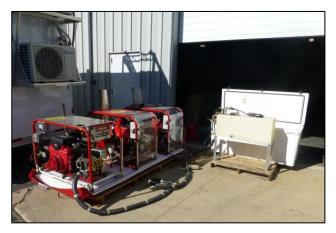
The IDDO Small Hot Water Drills (SHWD) use hot water to create shallow holes in the ice. They are non-coring and are typically used to produce holes 100-200 mm in diameter down to a maximum practical depth of 60. Primary use is for shot holes for seismic work, but they have also been used for access holes through a thin ice shelf. These drills are transportable by light aircraft and helicopter. These systems are typically operated by investigators without assistance from IDDO
