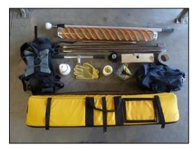
depth to which hand augers can be used without power assistance (see Sidewinder section) is approximately 20 m.
