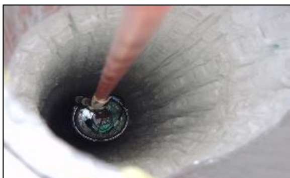
A Digital Optical Module (DOM) is lowered into a hole in the ice at Amundsen-Scott South Pole Station as part of the IceCube project. IceCube will search for neutrinos from distant astrophysical sources. Photo credit: Ethan Dicks, National Science Foundation.
