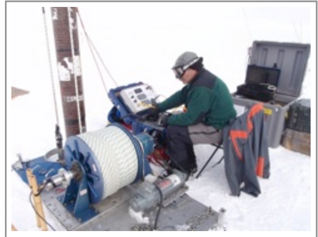
Terry Gacke drilling an ice core in Greenland with the 4-Inch drill. Photo: Bob Hawley
