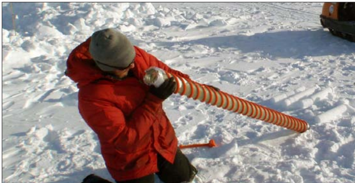
Josh Goetz field tests a new hand auger design at WAIS Divide. Photo courtesy of Steffen Bo Hansen.
