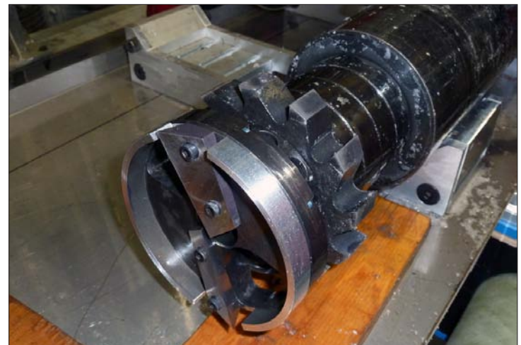
The Replicate Coring System's milling head with cutters. Photo courtesy of Jay Johnson.
