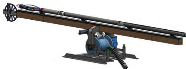
The tilting tower and winch, shown above, is a brand new design by IDDO using a lot of new technological advances from the DISC Drill. The tower is modular allowing it to fit inside a Twin Otter, or similar sized, aircraft.
