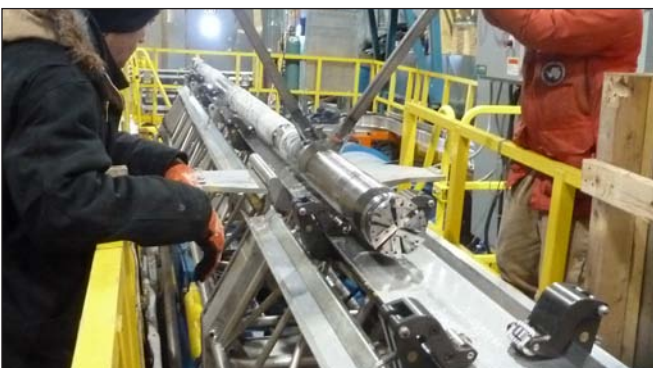
The replicate sonde with the milling head is shown. Photo: Chris Gibson, UW-Madison, IDDO
