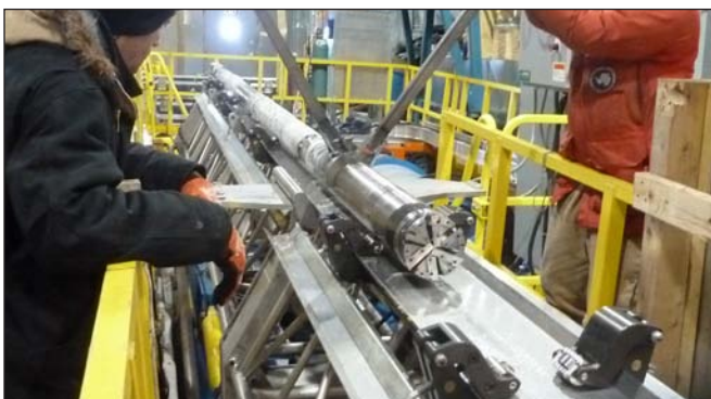
The replicate sonde with the milling head is shown. Photo: Chris Gibson, UW-Madison, IDDO
