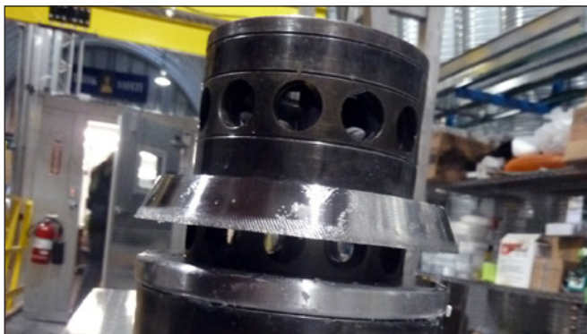
The broaching head of the replicate sonde is shown. Photo: Chris Gibson, UW-Madison, IDDO
