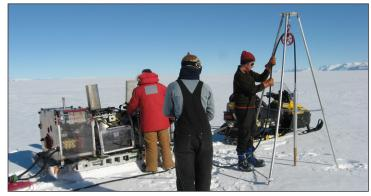
Drilling seismic shot holes with the portable hot water drill on Beardmore Glacier. Photo: Maurice Conway.
