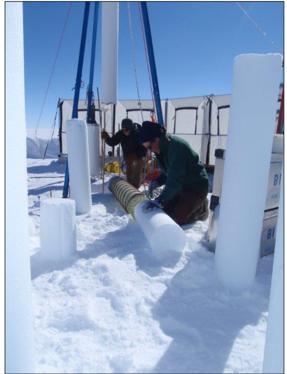
Blue Ice Drill firn coring testing in Greenland. Photo: Tanner Kuhl
