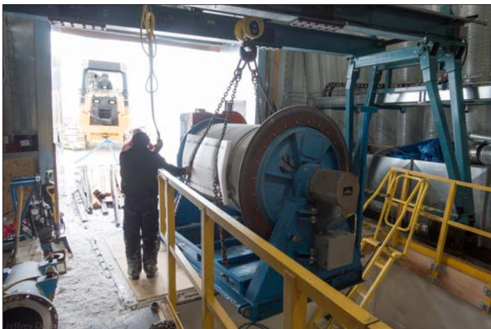
The DISC Drill winch is lifted out of the winch pit. Credit: Jeffrey Donenfeld
