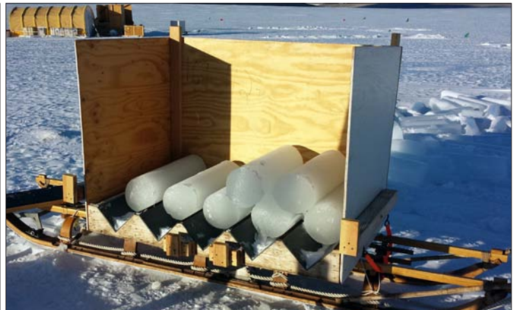
View of the sled used to transport the large-diameter ice cores. Credit: IDDO
