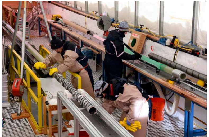
Science team members work in the South Pole Ice Core drill tent during the 2014-2015 field season cleaning the Intermediate Depth Drill and measuring ice cores. Credit: Peter Rejcek, National Science Foundation.
