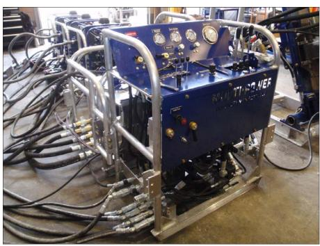
The control panel for the ASIG Drill system.
