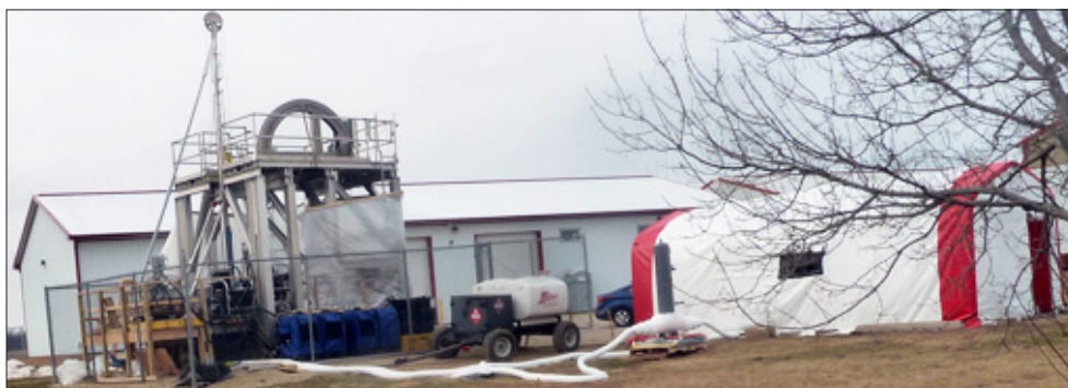
(Left) The 10-inch (0.25 meter) ice column being formed in the casing insert. (Right) The ASIG Drill test site at the UW PSL. At left, the ASIG Drill rig sits on a wooden deck with hydraulic engines in blue covers and wire-line tower visible above pre-existing aluminum platform; at center, a 500 gallon (1890 L) diesel wagon; at right, the drill tent housing the chiller; frosted glycol supply hoses visible in foreground. Credit: Chris Gibson
