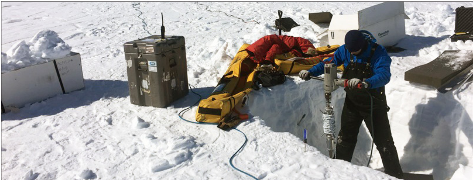
PI Erich Osterberg drills with the IDDO Hand Auger & Sidewinder system in Greenland. Credit: GreenTrACS Team/Dartmouth College
