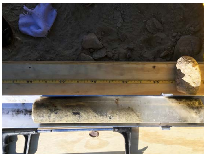
A mixed-media core consisting of ice, silt and rock collected with the Winkie Drill in Ong Valley, Antarctica. Credit: Grant Boeckmann
