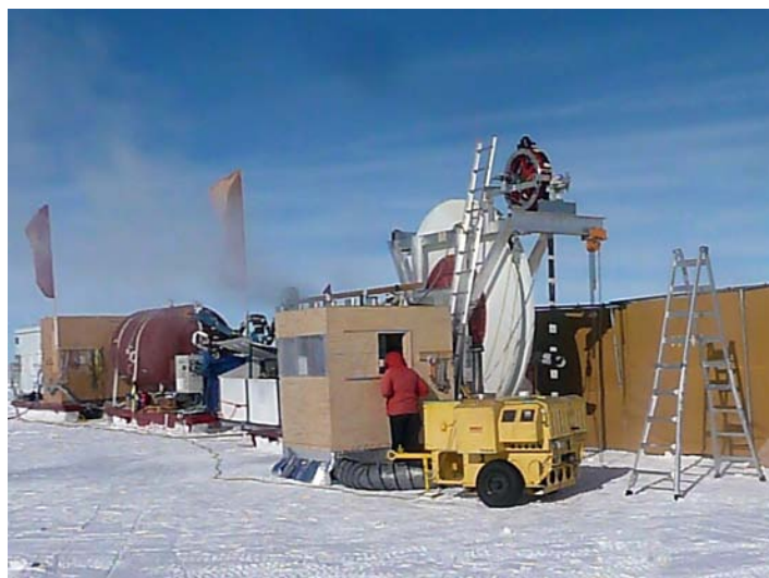
ARA hot water drilling at South Pole. Credit: Chris Gibson
