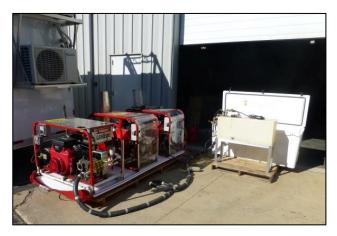
The IDP Small Hot Water Drills (SHWD) use hot water to create shallow holes in the ice. They are non-coring and are typically used to produce holes 100-200 mm in diameter down to a maximum practical depth of 60 m. Primary use is for shot holes for seismic work, but they have also been used for access holes through a thin ice shelf. These drills are transportable by light aircraft and helicopter. Feedback on system performance is continuously collected from users of the system.
