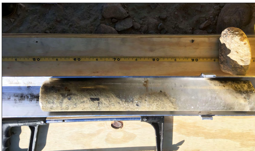
During the 2017/18 Antarctic field season, Jaakko Putkonen & team used the Winkie Drill to recover ancient ice buried under sediments in the Ong Valley floor of Antarctica. Some sections of the ice cores were clear clean ice, others were full of rocks & sediment. Credit: Grant Boeckmann.
