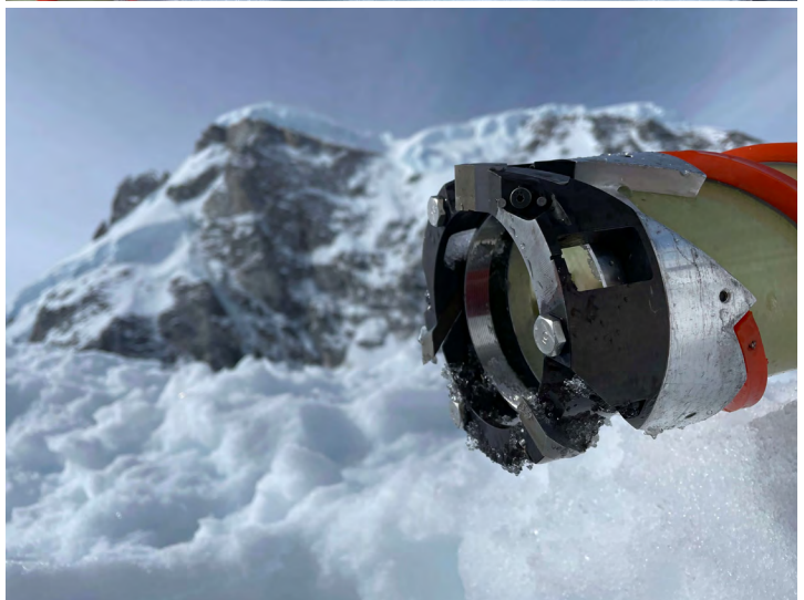
(Top) Julia Andreassen logs a core drilled with the IDDO Hand Auger at Combatant Col, British Columbia, Canada. Credit: Peter Neff. (Bottom) A close-up view of the IDDO Hand Auger cutter head. Credit: Peter Neff.
