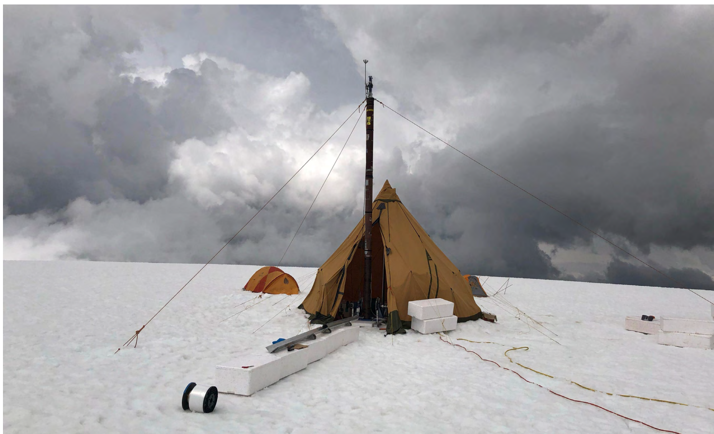
The Electromechanical Drill on the Quelccaya Ice Cap, Peru. The Electrothermal Drill was chosen because it works well in locations where the ice is close to its pressure melting point. In such situations, the more common electromechanical drills are at risk of getting stuck from melting and refreezing of the surrounding ice. The Electrothermal Drill uses a ring-shaped heating element in the coring head to melt an annulus around the ice to be cored, rather than shaving it away with cutters like electromechanical drills. Credit: Elliot Moravec.
