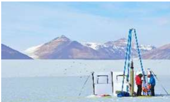
Caption: A large-volume ice core drilled on the Taylor Glacier ablation zone, Antarctica. Bubbles in the ice at the site contain evidence of ancient atmospheric composition. The Blue Ice Drill is an easily-transportable drill capable of retrieving quality firn cores of approximately 9.5 inches in
