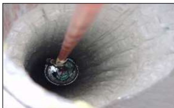
A Digital Optical Module (DOM) is lowered into a hole in the ice at Amundsen-Scott South Pole Station for the IceCube project. IceCube detects neutrinos from distant astrophysical sources. Photo credit: Ethan Dicks, National Science Foundation.
