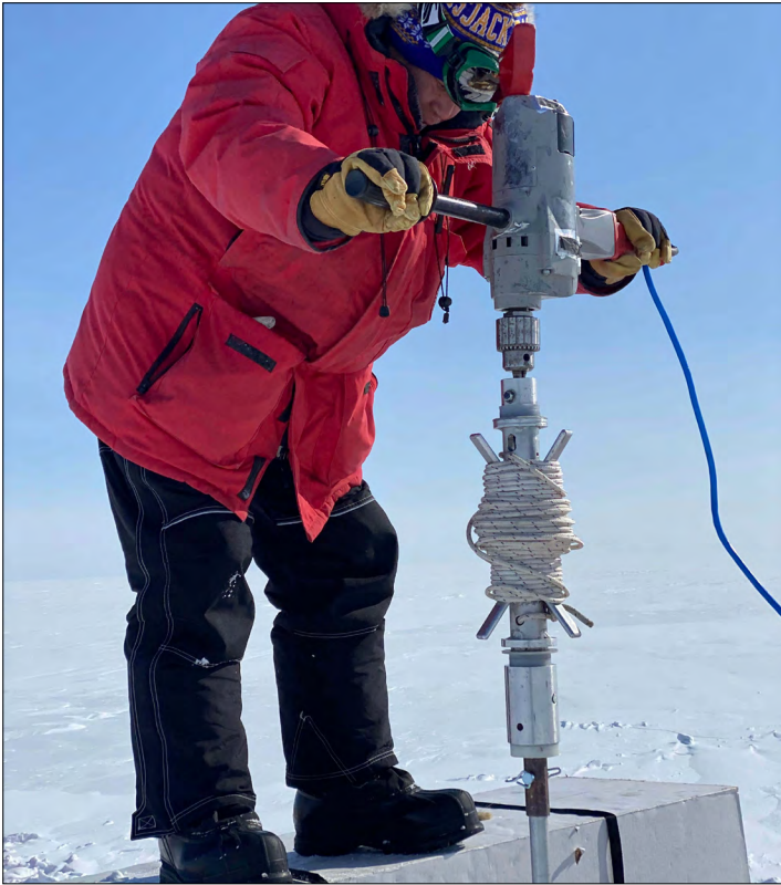
(Left) Jihong Cole-Dai uses the Sidewinder (with the IDDO Hand Auger) to drill a firn core at Summit, Greenland. Credit: Nathan Chellman, DRI. (Right) Jihong Cole-Dai logging a firn core at Summit, Greenland. Credit: Nathan Chellman, DRI.
