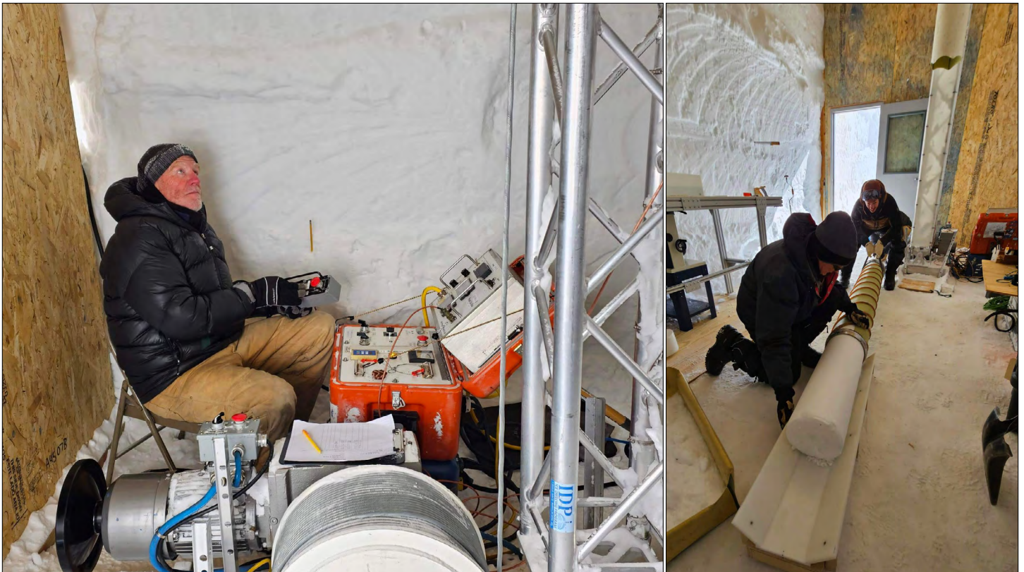
(Left) IDP Driller Mike Jayred operates the Blue Ice Drill at Summit, Greenland, in support of PI Nathan Chellman's project. Credit: Nathan Chellman, DRI. (Right) PI Nathan Chellman's science team pushes a core out of the barrel of the Blue Ice Drill. Credit: Nathan Chellman, DRI. To read fieldwork updates from this project, visit https://storymaps.arcgis.com/stories/a0d9664d399b47c585c5485265509deb .
