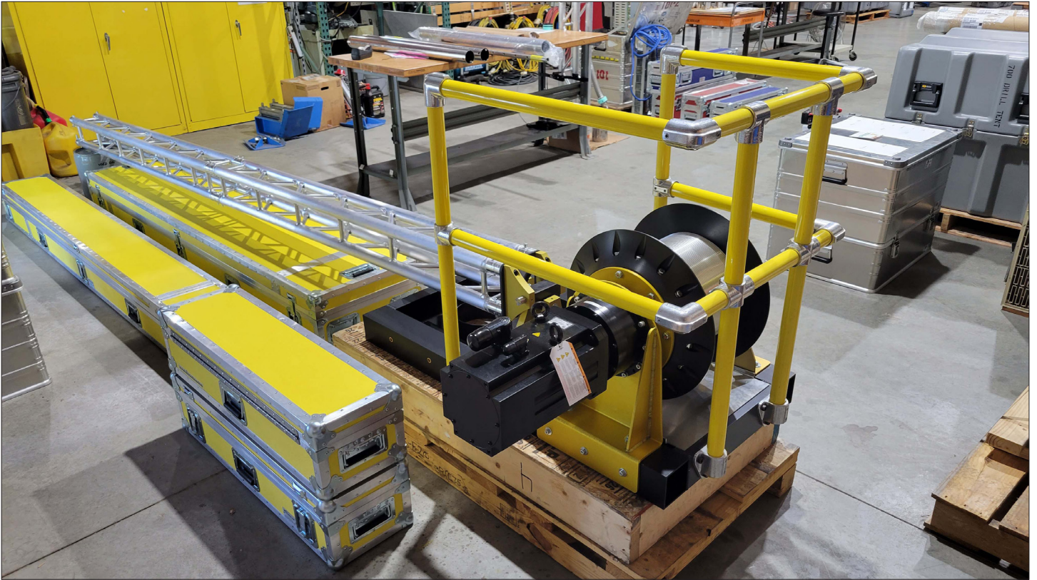
The new 700 Drill winch and tower assembled at the IDP facility in Madison, WI. Credit: Jay Johnson.
