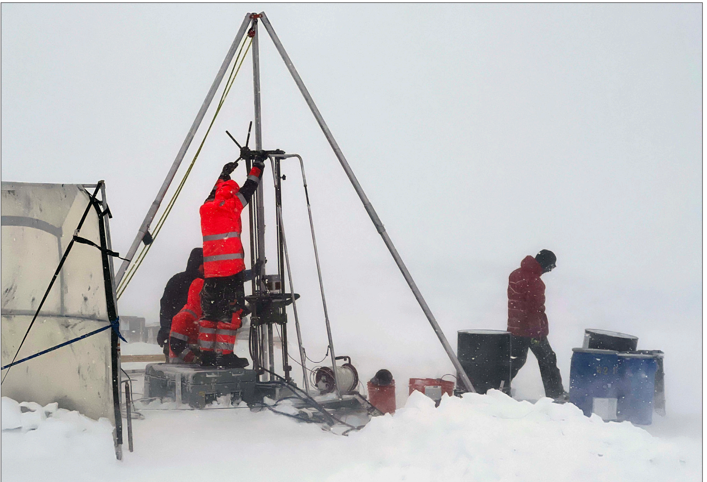
IDP Driller Rubin Harmon operates the Winkie Drill in windy conditions in northwest Greenland. Credit: Jason Briner.
