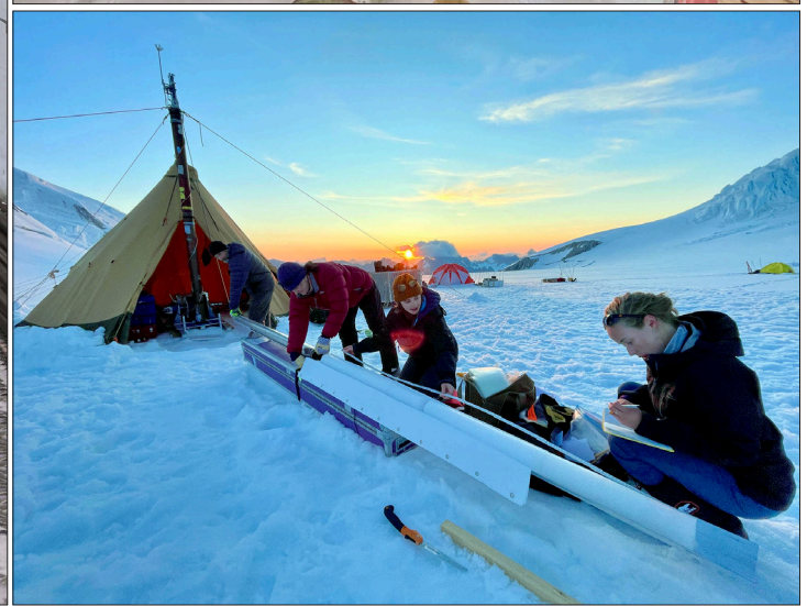
(Left) IDP contract rock drill rig operator Richard Erickson operates the IDP ASIG Drill for the GreenDrill project. Credit: Tanner Kuhl. (Right, top) PI Nathan Chellman's team at Summit Station with a large-diameter ice core drilled with the IDP Blue Ice Drill. Credit: Mike Jayred. (Right, bottom) Drilling on Mt. Waddington in British Columbia, Canada, with the IDP Thermal Drill. Credit: Peter Neff.
