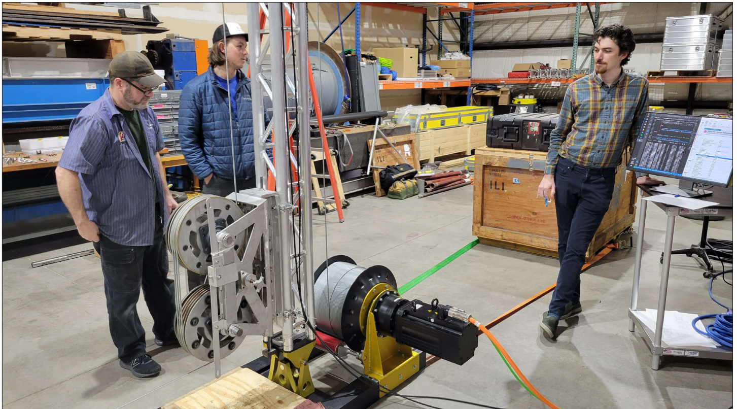
(Right) Electronics testing of the 700 Drill's sonde. Credit: Umberto Stefanini. (Bottom) IDP engineers spool the 700 Drill's cable onto the winch. Credit: Jay Johnson.
