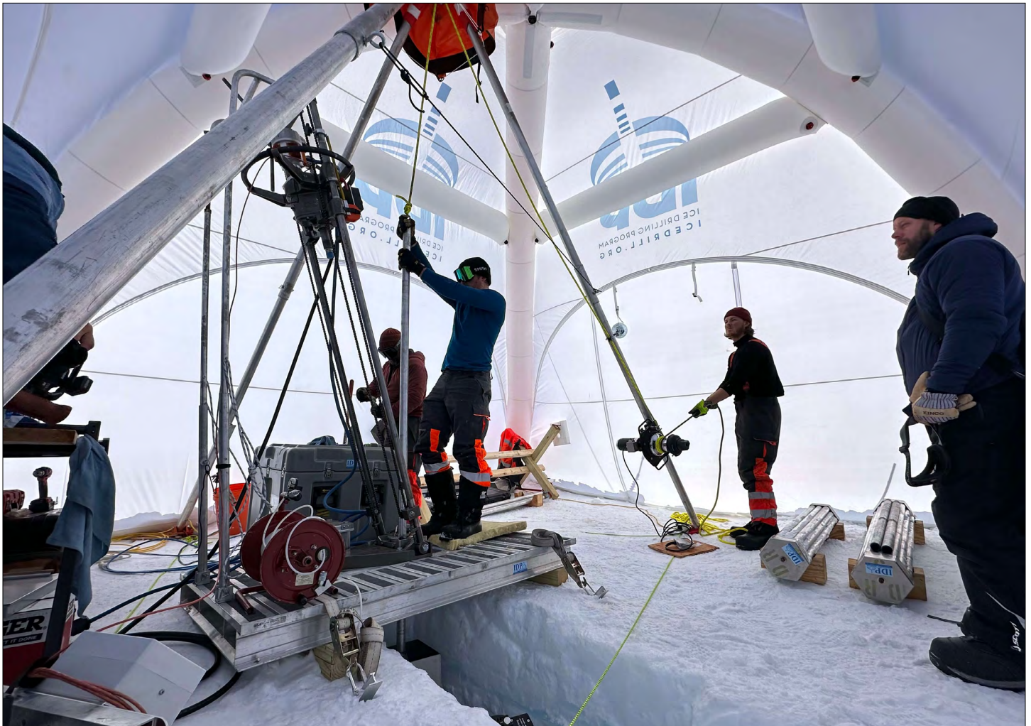
IDP Winkie Drill operations in a new inflatable Axion tent in NE Greenland in support of the GreenDrill project. Credit: Allie Balter-Kennedy.
