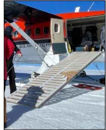
Aircraft cargo ramp designed by IDP
