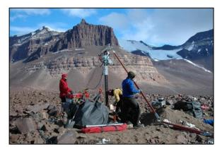
motor mounted to a tower. Drill penetration is controlled by a feed system on the drill tower to account for varying ice conditions. The drill produces 76-mm (3-inch) diameter cores a few tenths of a meter long. It was tested and used to collect scientific samples in Beacon Valley during the 2006-2007 Antarctic field season and again, after repair and modification, in the 2008-2009 and 2009-2010 field seasons. It has not been used since.
