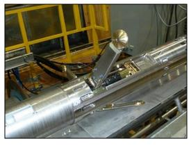
to obtain additional volumes of ice samples at selected intervals, termed replicate coring, addresses these concerns and adds value to the scientific return from ice coring. It is important that the taking of replicate cores doesn't compromise other scientific activities, in particular borehole logging.
