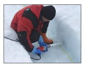
**2.1.1 Chipmunk Drill** – The smallest drill in the IDDO inventory, it is a hand-held, motor driven coring drill that collects 2-inch diameter cores in solid ice. It has two barrels, one 15 cm long and one 50 cm long. The drill has been used on one funded project (for which it was designed) at Pakitsoq, West Greenland, in 2003 and 2004, for exploratory work at the South Pole in 2013 and for several demonstrations of ice coring for the public in the U.S.
