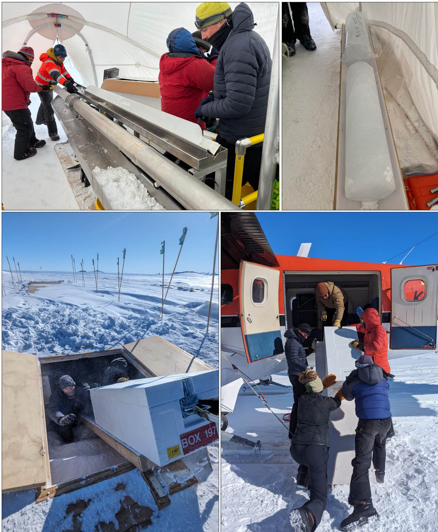
(Top) A run of ice from the smaller-diameter Shallow Wet Drill (left) and large-diameter Blue Ice Drill (right) drilled during the 2025/2026 field season at Allan Hills, Antarctica. Credit: IDP. (Bottom) Core boxes being pulled out of the core storage trench (left) and loaded onto a Twin Otter (right) at Allan Hills, Antarctica, during the 2025/2026 field season. Credit: Matthew Kippenhan/ASC.
