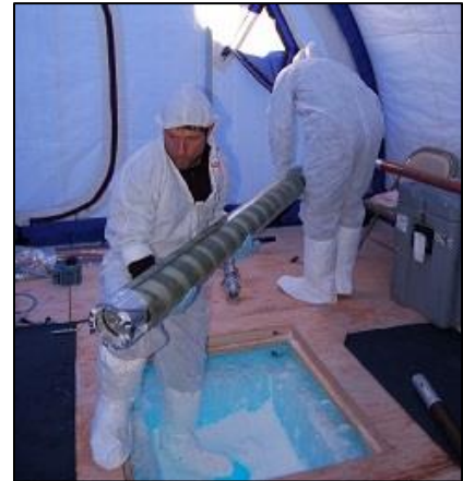
Prairie Dog system used with a Hand Auger
