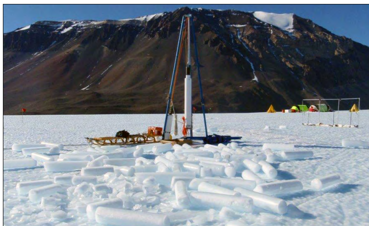
The Blue Ice Drill is designed to collect large volumes of ice (9.5-inch diameter cores) in a short period of time. The large volumes of ice enable ultra-trace gas measurements, such as the carbon-14 of methane, that historically have been precluded by sample size limitations of ice cores. Photo courtesy of Tanner Kuhl.
