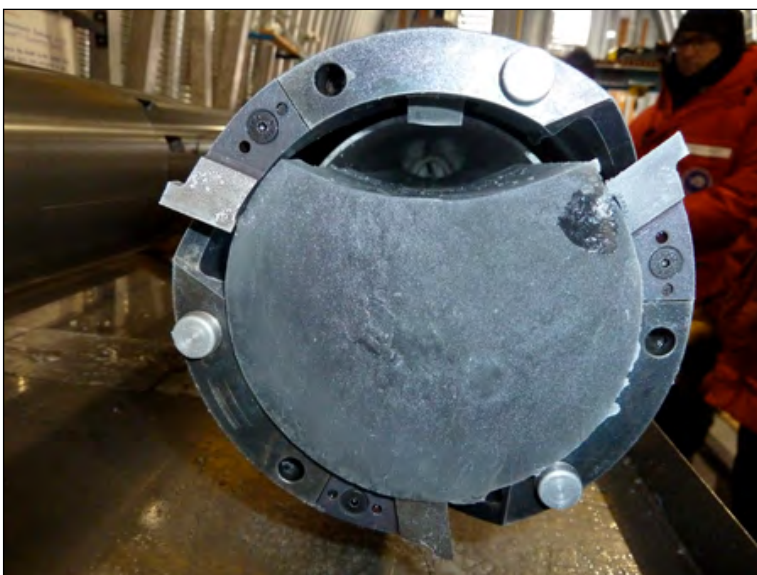
The coring head with the first replicate ice core ever taken from the "uphill" side of an ice core borehole is shown. Photo: Jay Johnson, UW-Madison, IDDO
