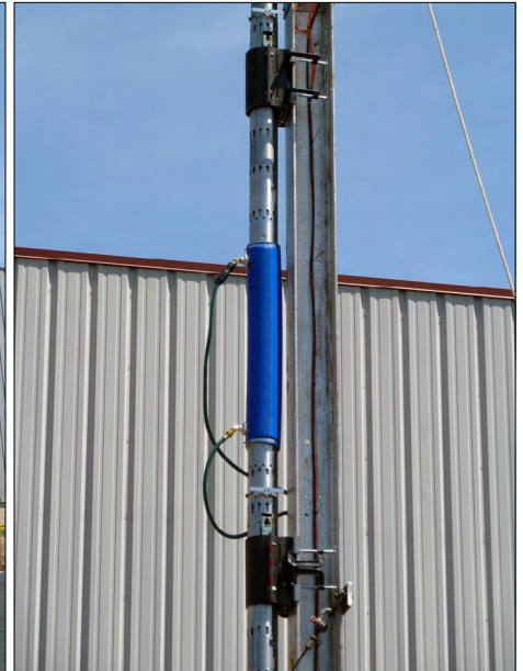
Replicate coring system testing in Madison, WI. Cooling jacket for replicate instrument section.
