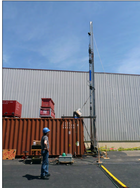
Replicate coring system testing in Madison, WI. Cooling jacket for replicate instrument section.
