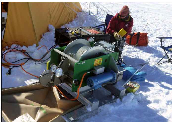
The new intermediate logging winch for logging boreholes up to 1500 meters deep.
