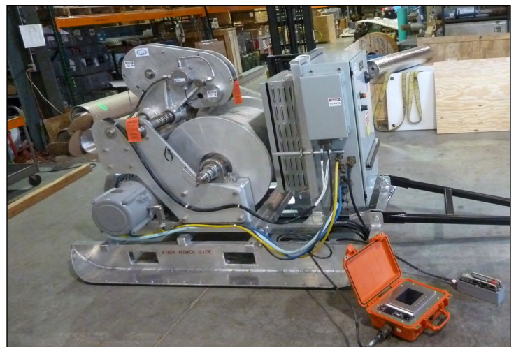
The new deep logging winch for logging boreholes up to 4000 meters deep.
