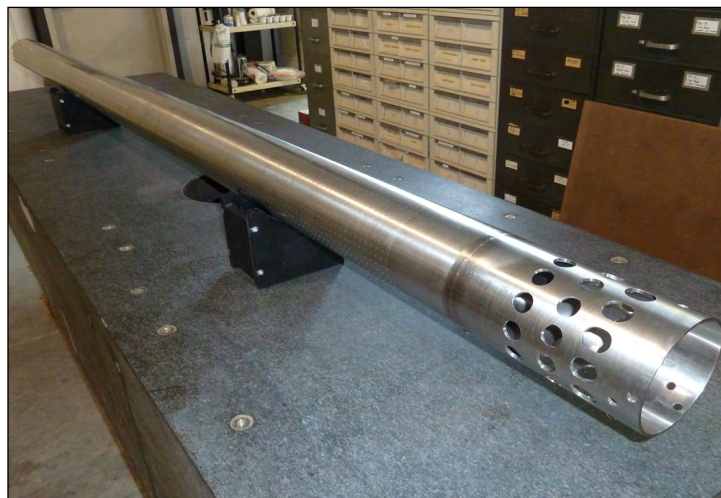
View of the Intermediate Depth Drill's chips chamber.
