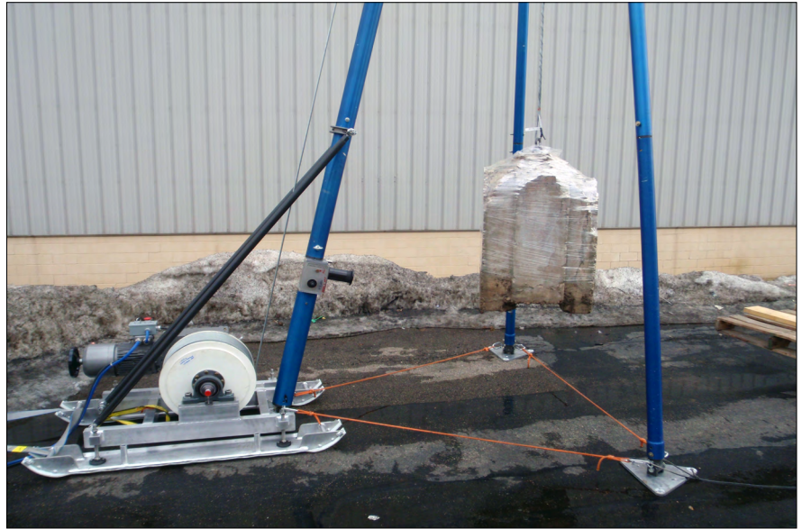
Blue Ice Drill – Deep winch and tripod assembly.
