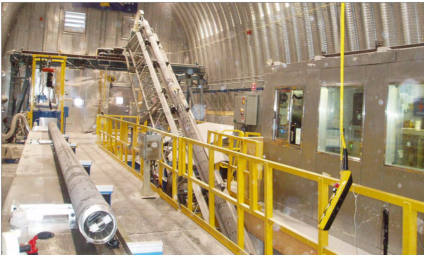
Image of the Deep Ice Sheet Coring (DISC) Drill at WAIS Divide, Antarctica. The DISC Drill is a tilting-tower electromechanical drill designed to cut and retrieve cores of ice 122 mm (4.8 inches) in diameter to depths of 4,000 meters. Photo Credit: Jay Johnson/IDDO.
