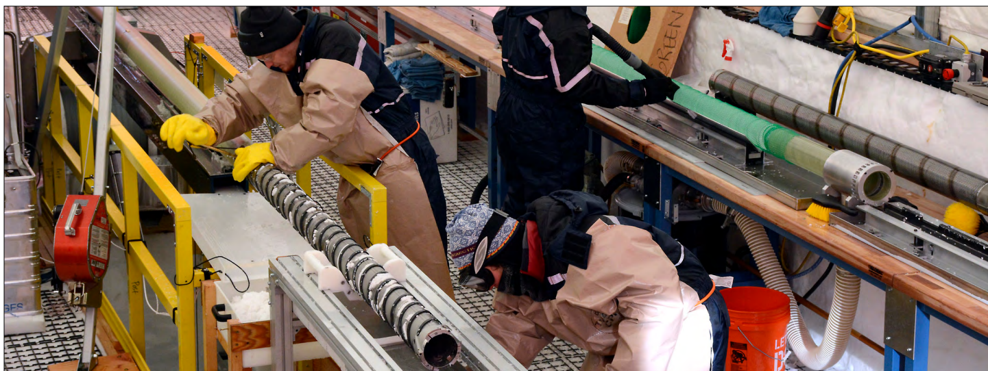
Science team members work in the South Pole Ice Core (SPICE) drilling tent cleaning the Intermediate Depth Drill and measuring ice cores. Credit: Peter Rejcek, NSF
