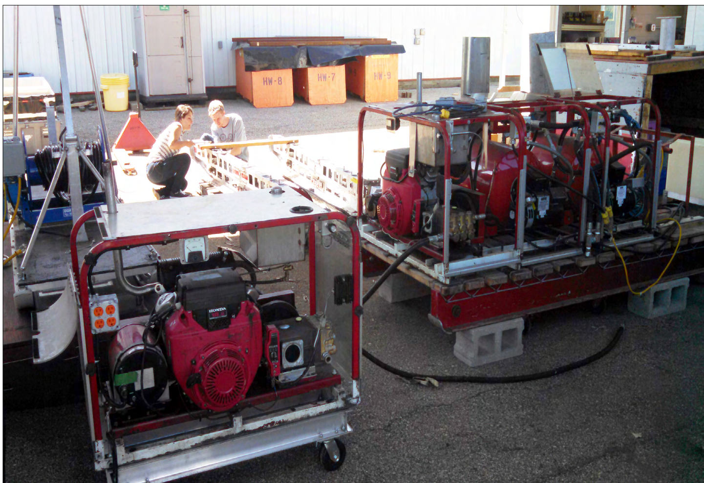
The Small Hot Water Drill set-up at PSL for testing/upgrade Credit: Terry Benson, UW Physical Sciences Lab
