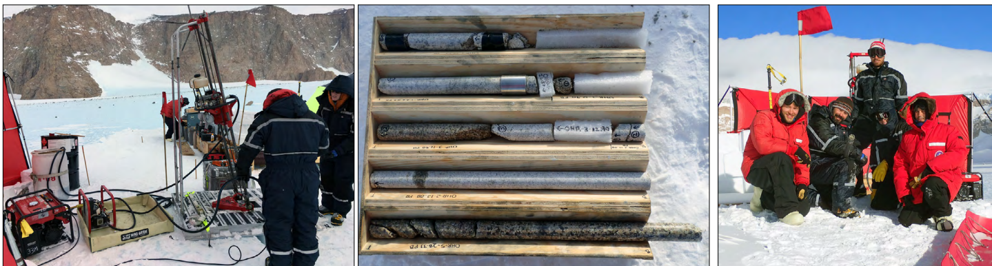
Left: The assembled Winkie Drill system at the Ohio Range. Credit: Grant Boeckmann. Middle: Packaged rock cores drilled with the Winkie Drill. Credit: Sujoy Mukhopadhyay. Right: The Ohio Range field team after their first successful rock core with the Winkie Drill Credit: Sujoy Mukhopadhyay.
