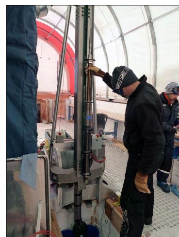
Laser dust logging of the SPICECORE borehole. Credit: Jay Johnson.
