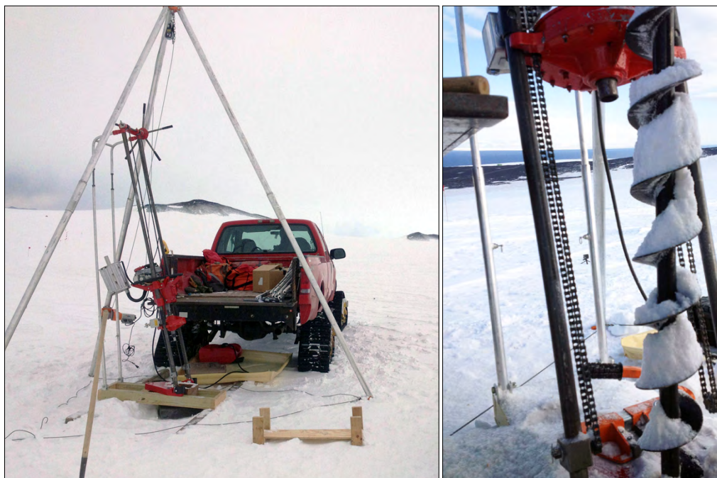
(Left) Winkie Drill testing near McMurdo Station, Antarctica, during February 2016. (Right) Winkie Drill with Kovacs auger attachments. Credit: IDDO
