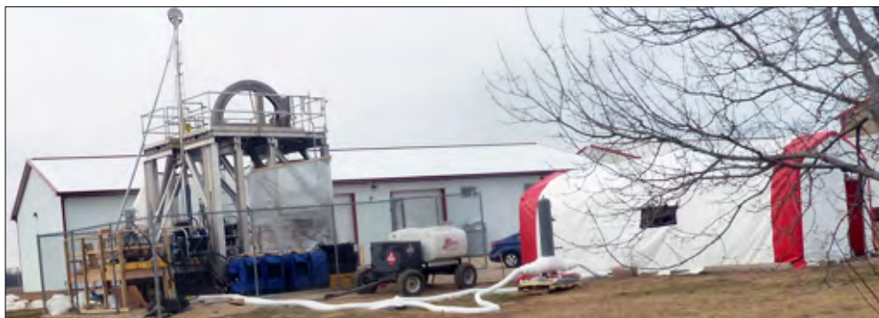
(Left) The 10-inch (0.25 meter) ice column being formed in the insert. (Right) The ASIG Drill test site at the UW PSL. At left, the ASIG Drill rig sits on a wooden deck with hydraulic engines in blue covers and wire-line tower visible above pre-existing aluminum platform; at center, a 500 gallon (1890 L) diesel wagon; at right, the drill tent housing the chiller; frosted glycol supply hoses visible in foreground. Credit: Chris Gibson
