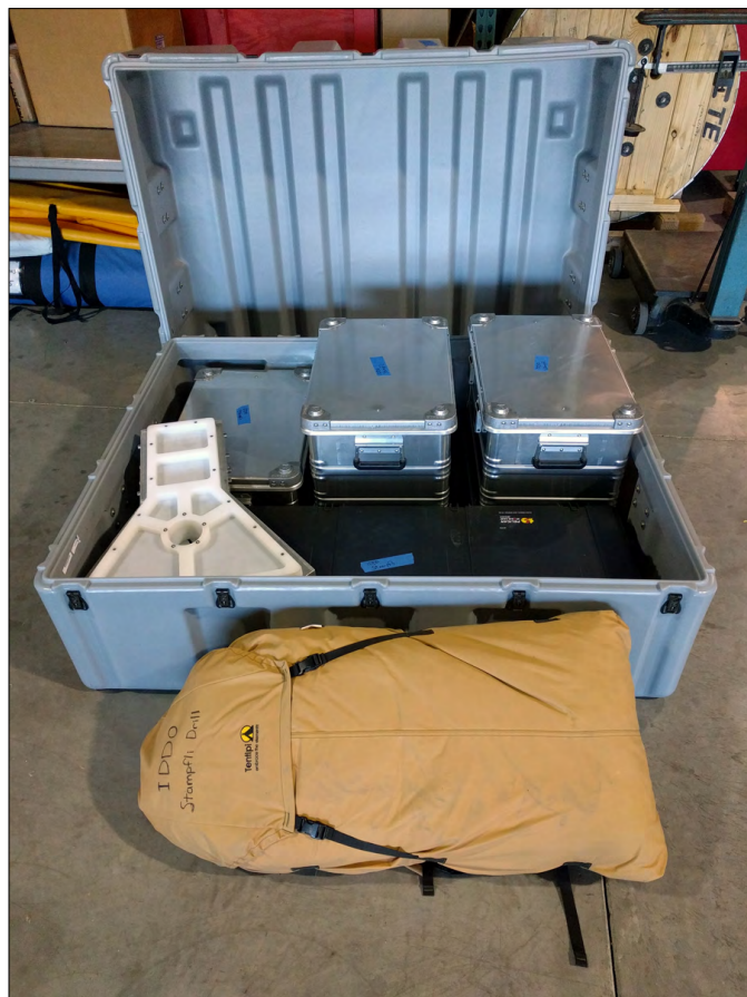
Left: IDDO driller Elizabeth Morton field testing the Stampfli 2-Inch Drill in Greenland. Credit: Michael Jayred. Right: The shipping crate for the Stampfli Drill. Also shown is the optional tent (inside the brown/tan bag), which also fits inside the shipping crate. Credit: IDDO
