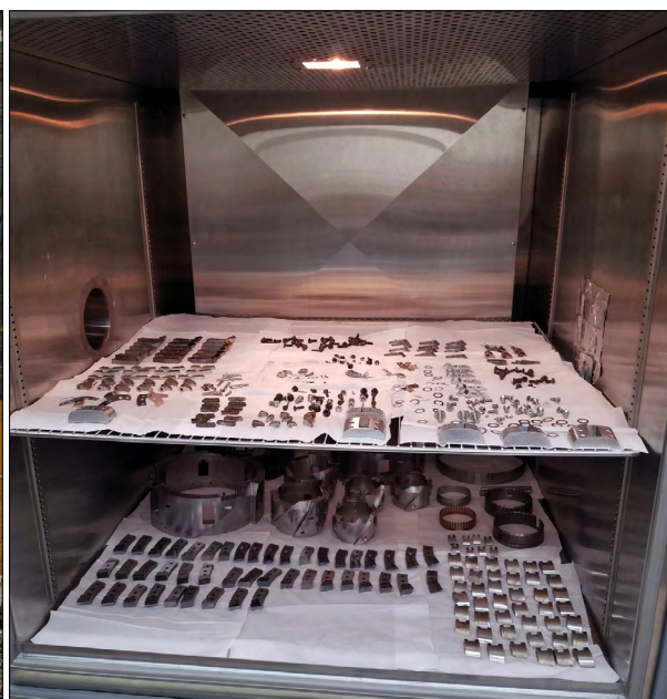
Left: Ultrasonic cleaning of cutters and other metal parts. Right: Baking of drill parts in a Tenney environmental chamber at 50 °C. Credit: Jay Johnson.
