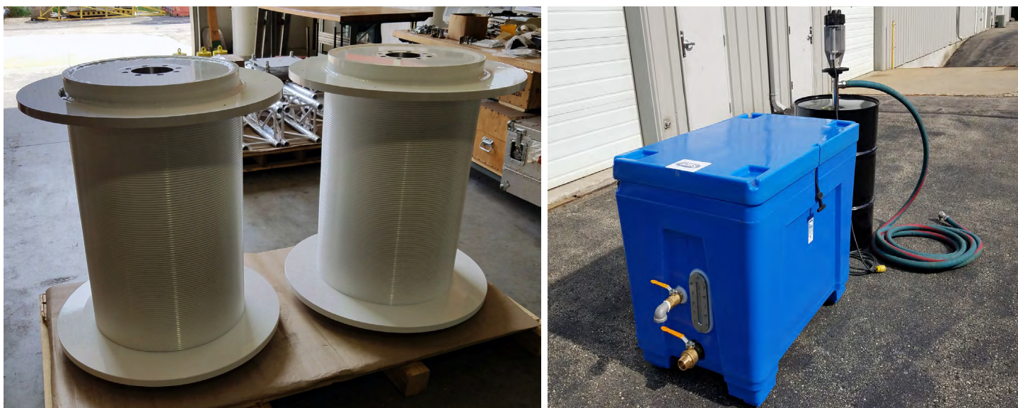
(Left) The Foro 3000 winch drums and (Right) chip melter tank and drill fluid drum pump. Credit: Jay Johnson
