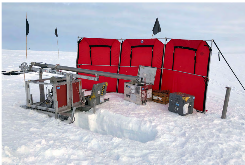
Badger-Eclipse Drill set up for access hole drilling to bedrock at Winkie Nunatak in the Hudson Mountains of Antarctica for the C-443 GHC project (PI Ryan Venturelli). Credit: Elliot Moravec
